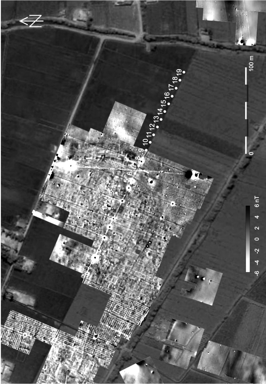
3. †Ezbet Machali. Magnetic map and location of vertical electrical soundings. Magnetic survey by fluxgate (in settled areas) and cesium (river bed deposits) magnetometers. Arrows mark long structures of undefined nature, paralleling the waterfront (see text). Prospection and data processing by T. Herbich and C. Schweitzer (© ÖAI).
